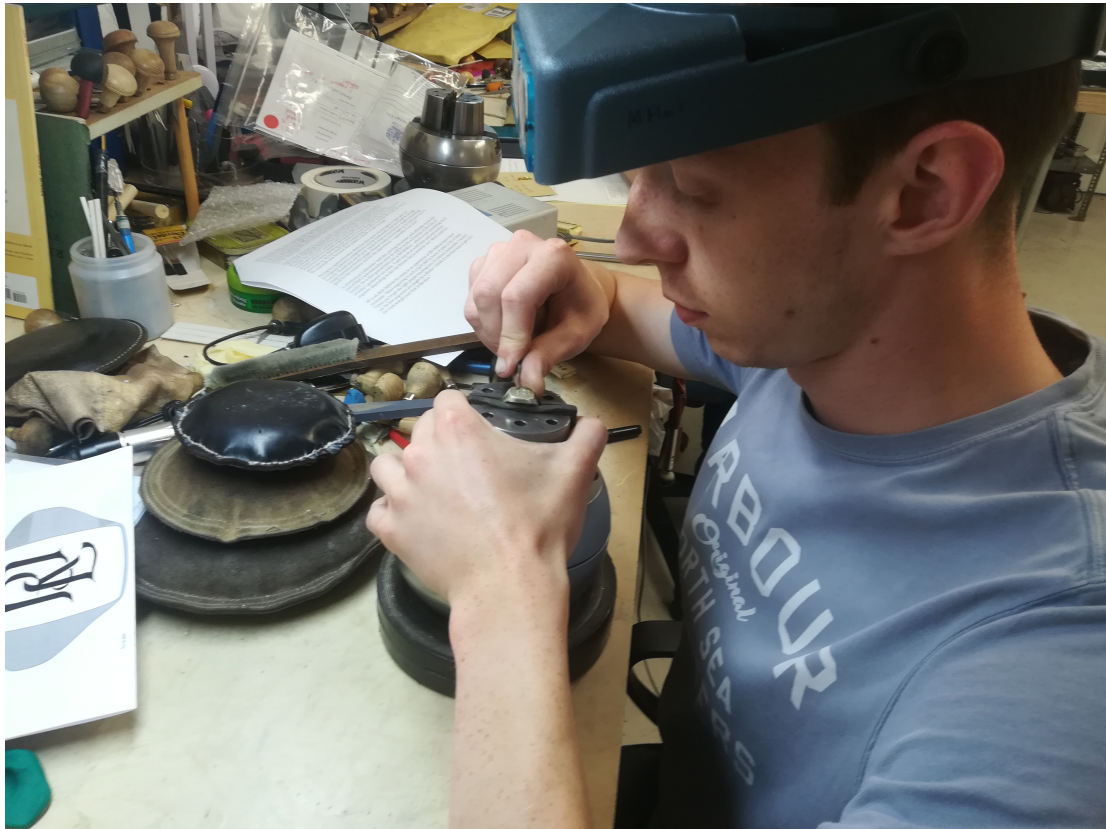
Matt using a flat engraving tool to seal engrave a monogram on a silver signet, copying a customer's artwork
